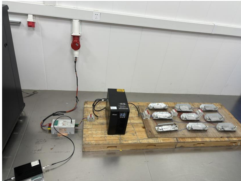
CONDUCTED SUSCEPTIBILITY TEST
