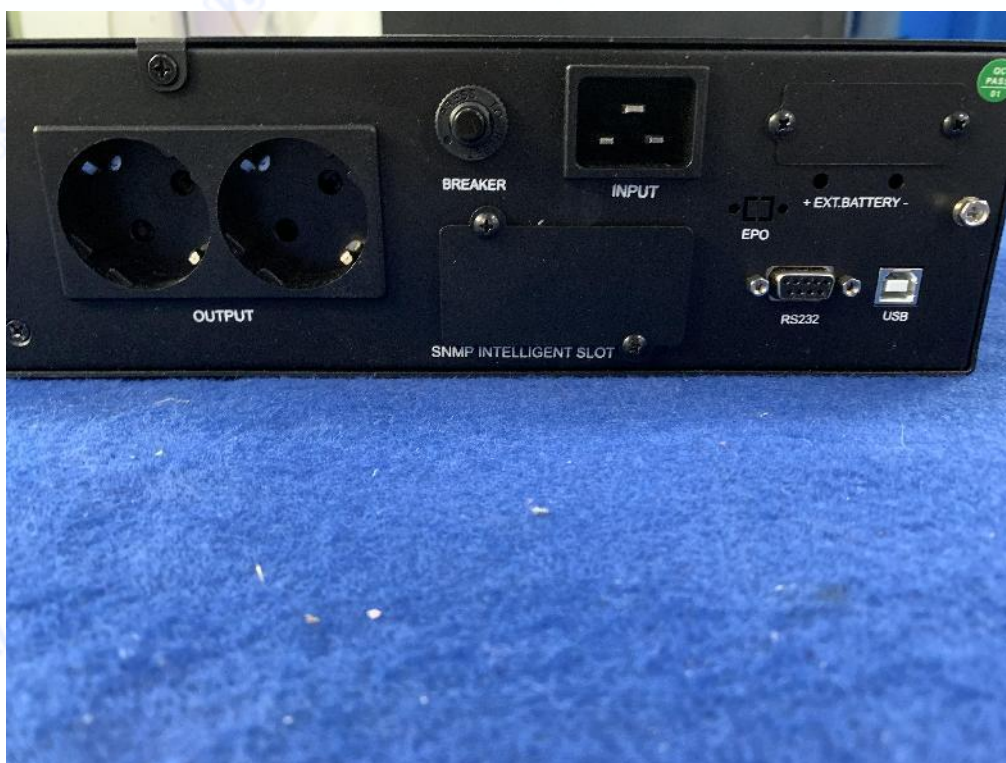
Photo 18: Socket and Appliance inlet view
